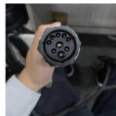
Connect the P1 interface of the navigation terminal ISOBUS wire harness (as shown below) to the agricultural implement wire harness interface, and connect the P4 interface to the CAN interface of the navigation terminal.
