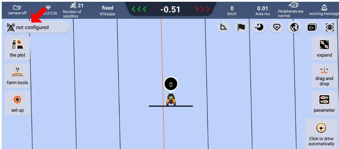
**1. On the main screen, click the “base station configuration” in the upper left corner to go to the differential setup page.**
